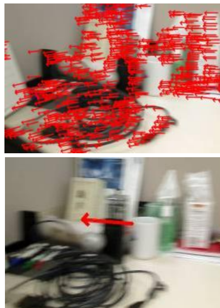
Fig 2. Example of optical flow field (top) and resulting overall optical flow 2D vector (bottom).
