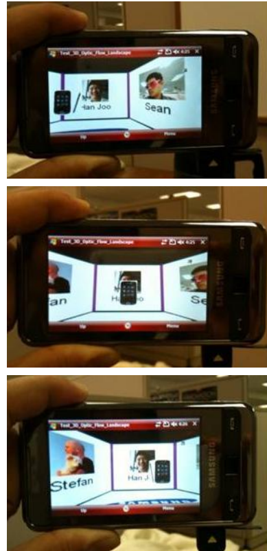
Fig. 7. Example of a sideways shifting motion, at a slow yet constant speed. This is detectable reliably with optical flow from an imager in parallel to the motion plane, but not reliably with inertial sensors alone.
